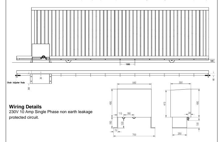
**PLEASE NOTE:** The specifications and suggested gate sizes will vary depending upon other variables such as friction of wheels, environmental factors e.g. wind loading, type of cladding and external influences which may assist or degrade the recommended gate sizes.
