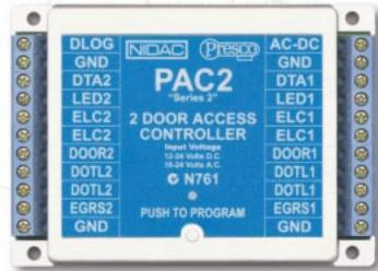
With the Presco" system the door controller and reader are separated, allowing the controller to do the code processing in a remote protected environment. The code is transmitted from the reader using only two wires, making installation simple and cost effective. The door controller and reader can be separated by up to 1 kilometer using low cost 4 core non-shielded cable!
